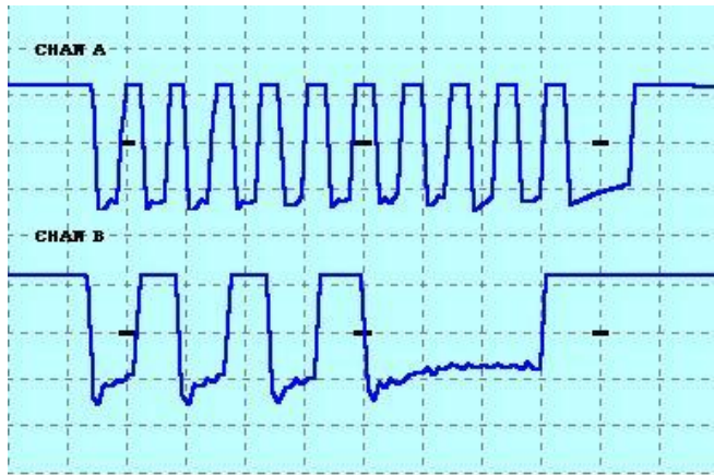
Figure 2: Scan code for the "Q" key (15h) being sent from a keyboard to the host (channel A - clock, channel B - Data).
